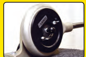
Step 5: Install proper die, insert hose assembly into the crimper and firmly push down on handle.
