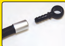
Step 3: Apply assembly lube to barbs and then push hose end into ProClassic hose.
